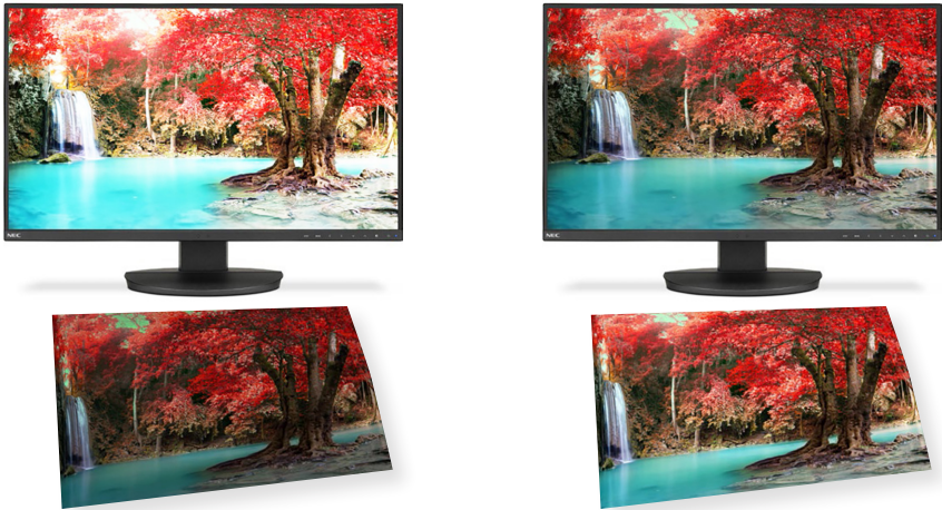
Fig. 8: Too bright display leads to a dark photo, a calibrated display leads to a faithful paper photo
