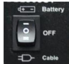
4. Connect power cable (use battery) and switch on the light (position „Cable“ or „Battery“). The color temperature and brightness can be adjusted in two ways:
