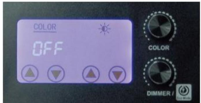
The color temperature range is 3000K - 8000K and the power output is from 0 - 100%. It reaches maximum power output in 5500K and 100%.
